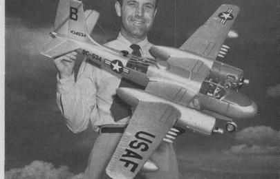
MORE THAN 700 man-hours of work went into building this handsome B-26 control line model made by Wally Boyes. He constructed the model from plans outlined in Air Trails magazine. Balsa wood, aluminum, brass, and some hard woods were used.
